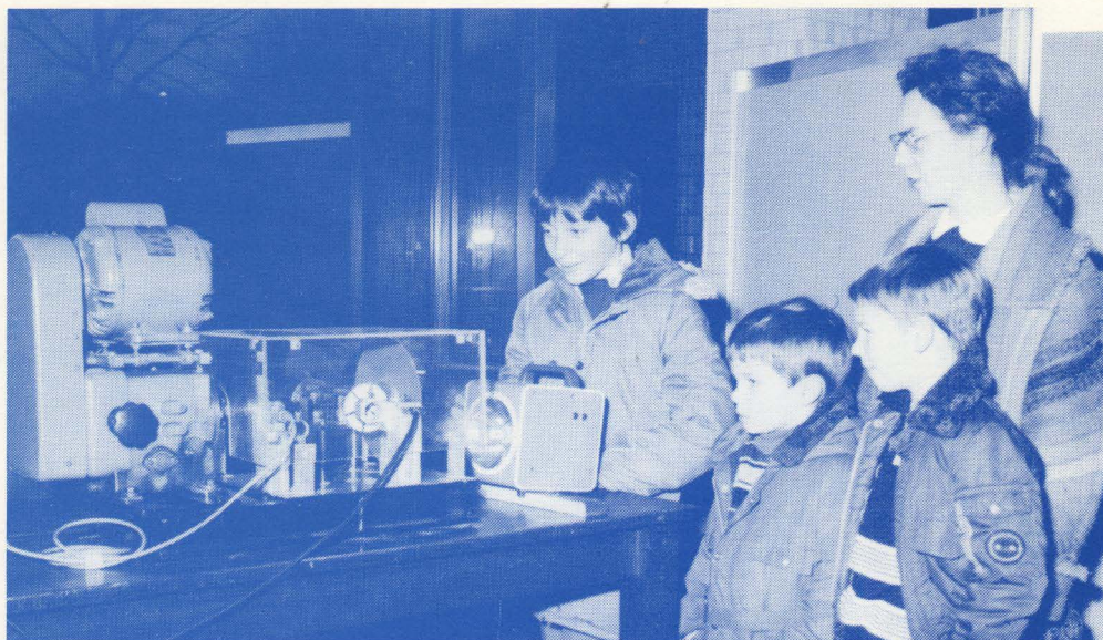
A moving machine can be 'frozen' with a stroboscope.
